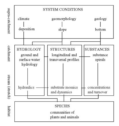
• Figure 2. Main structure of the 5-S-model with key factors and functional aspects (adapted from Verdonschot et al., 1998).
